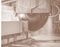
Fig. 3. The cutting of a stone block.
