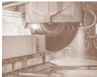
Fig. 3. The cutting of a stone block.
