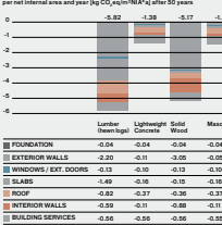
Fig. 07 THE GARDEN HOUSE: EMBODIED EMISSIONS FOR PRODUCTION, REPLACEMENT, DISPOSAL IN RELATION TO GLOBAL WARMING POTENTIAL (GWP) per net internal area and year [kg CO 2 eq/m 2 net internal area after 50 years]
